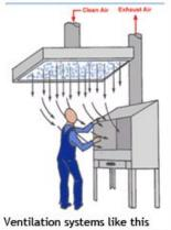
Ventilation systems like this one push and pull lead fume or dust away from the worker's breathing zone. Courtesy of OSHA
